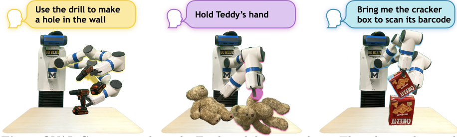
Fig. 1. OVAL-Grasp at work on the Fetch mobile manipulator. The robot understands which parts of the object it should grasp and which parts should be avoided to fulfill the given tasks described by language.
